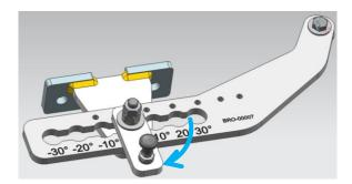
4. Place the machine at the requested orientation using the marking
