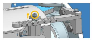
3. Place the machine at the requested orientation using the marking
