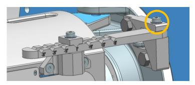
2. Unscrew the screw allowing the index to be lifted up (do not remove the screw )
