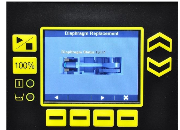
Figure 3 – Full In diaphragm replacement screen
