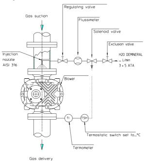
Thermometer TI have to regulate the water amount by the solenoid valve in order to mantain the discharge temperature T2 to the velue indicated at page 4. Thermostat TSH set at 145°C have to intervene to stop the blower in case of cooling circuit malfunctioning.
