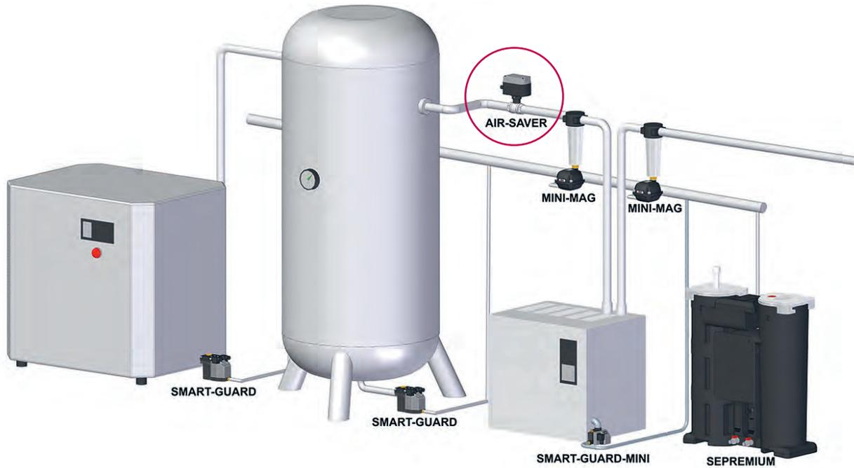
The AIR-SAVER typically gets installed after the receiver (air tank). Once closed, it retains the compressed air built up in the receiver and ensures that the compressor does not run unnecessarily during moment when it is not required.
