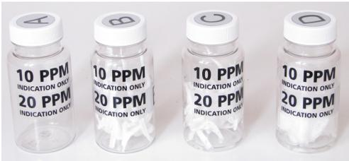
4. Shake the condensate (0,5L) and then fill all four test bottles with condensate (approx. 100ml each).
