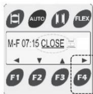
9. Choose the desired setting (OPEN or CLOSE) by pressing F2(▼) and F3(▲) to scroll down and up.
