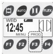
2. To **delete** a setting, choose the desired day and time by pressing F2(▼) or F3(▲) to scroll down and up. Press F4('EDIT') to select.
