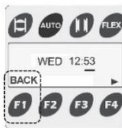
12. a) The units' VALVE OPEN AND CLOSE TIMES are pre-programmed to OPEN THE VALVE at 6.00 and CLOSE THE VALVE at 18.00, from Monday to Friday. If these pre-programmed VALVE OPEN AND CLOSE times suit your application, the unit is now set and ready for use.
