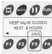
9. 'FLEX with an arrow pointing at the valve status indicator and remaining time' will now flash on the HOME screen, indicating the timer is now in FLEX FUNCTION. The background color of the display will turn red.
