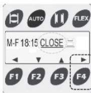
19. Choose the desired valve 'OPEN' or 'CLOSE' setting by pressing F2(▼) and F3(▲) to scroll down and up.
