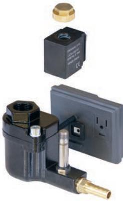
Servicing the SMART-GUARD-MINI could not be easier. The drain comes apart by unscrewing two screws. You lift the coil from the valve stem and you have direct access valve assembly.
