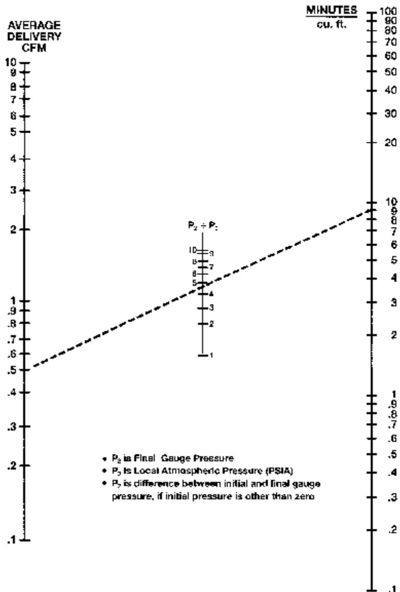
**EXAMPLE:** How much time is required to pressurize a 2 gallon volume from 0 to 75 PSIG using a 607CA22?
