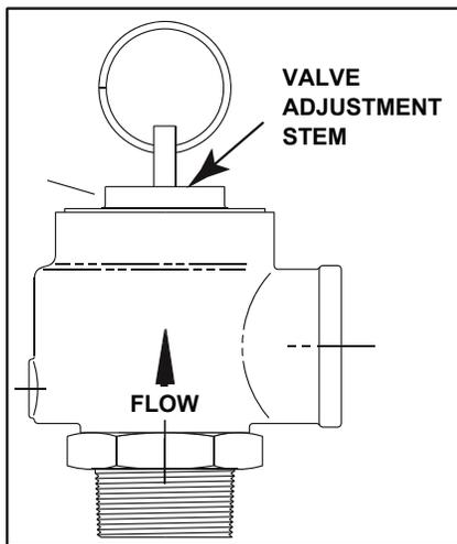
Figure 5-1 – Pressure Relief Valve Detail
