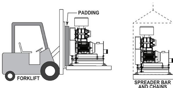
Figure 4-1 – Proper handling and lifting procedure.
