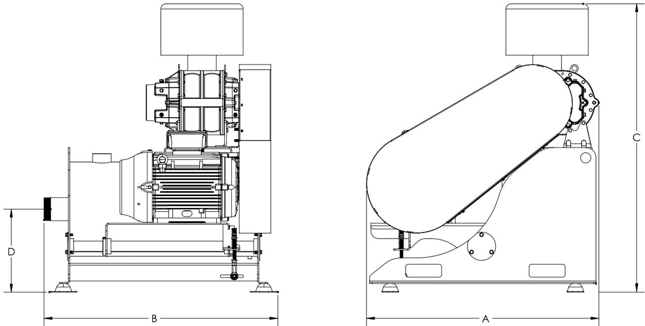
Figure 4-2 – MD20 Blower Package Dimension Drawing
