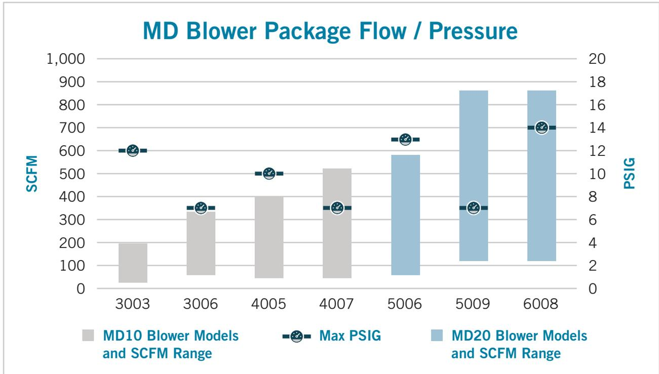
Figure 3-1 – MD Blower Package Flow / Pressure Chart
