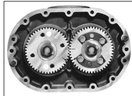
Figure 11 - Timing marks advanced 3 teeth (Reference marks aligned)
