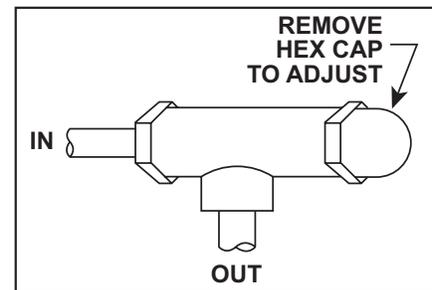
Figure 5 - Pressure Relief Valve
