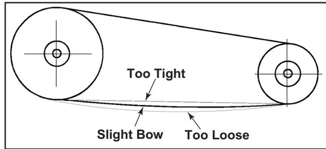
Figure 6 - General appearance of a V-Belt drive
