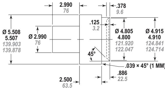
FIGURE 16 — ALIGNMENT TOOL FOR DRIVE SHAFT BEARING
