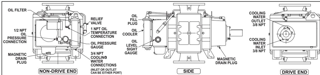
Figure 4 - Location of oil fill, drain plugs, level gauges and cooling connections
