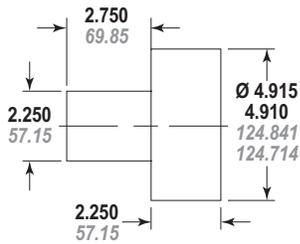
FIGURE 14 — BEARING INSTALLATION TOOL
