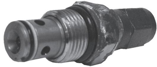
Figure 5-5 – Oil Pressure Adjustment Hex Cap
