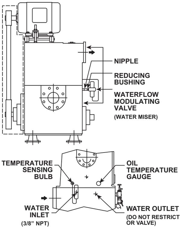
**NOTE: Water inlet and outlet are on the opposite side on the KT-150.**
