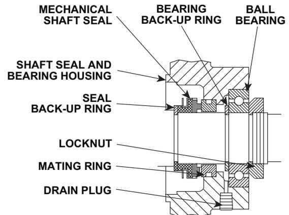
Figure 8-2 – KT-150 Shaft Seal and Bearing Housing
