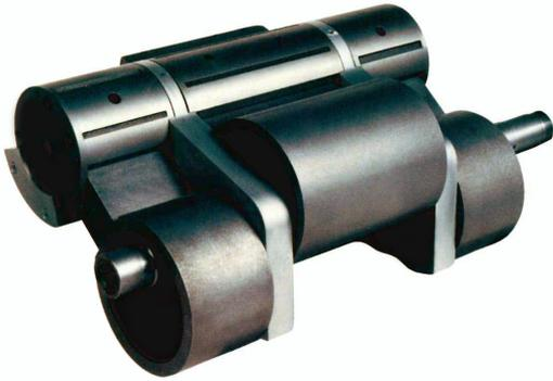
Figure 4-2 – Triplex Arrangement
