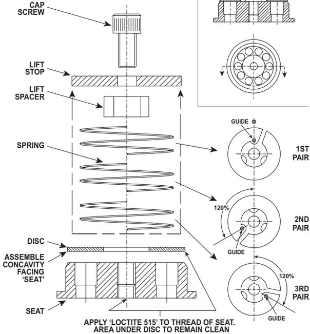
Figure 8-1 – Discharge Valve
