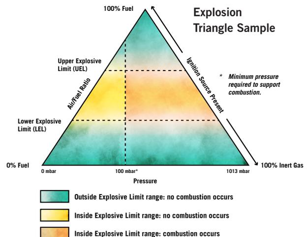
The blower or booster is intended to internally handle explosive gas mixtures up to the critical gas combustion pressure of approximately 100 mbar. This pressure varies by gas type. All product selections are required to be evaluated through MD-Kinney's VBxpert Portal sizing software prior to quotation. For pressures greater than 100 mbar ATEX Internal classification is not supported.
