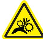
Internal and external rotating parts of the blower and driving equipment can produce serious physical injuries. The blower should never be run with the inlet or discharge piping removed. If it becomes necessary to inspect the rotating parts of the blower or to change V-belts, be absolutely sure that all power to the motor controls has been shut off, the motor controls are locked out, and properly tagged before proceeding.
