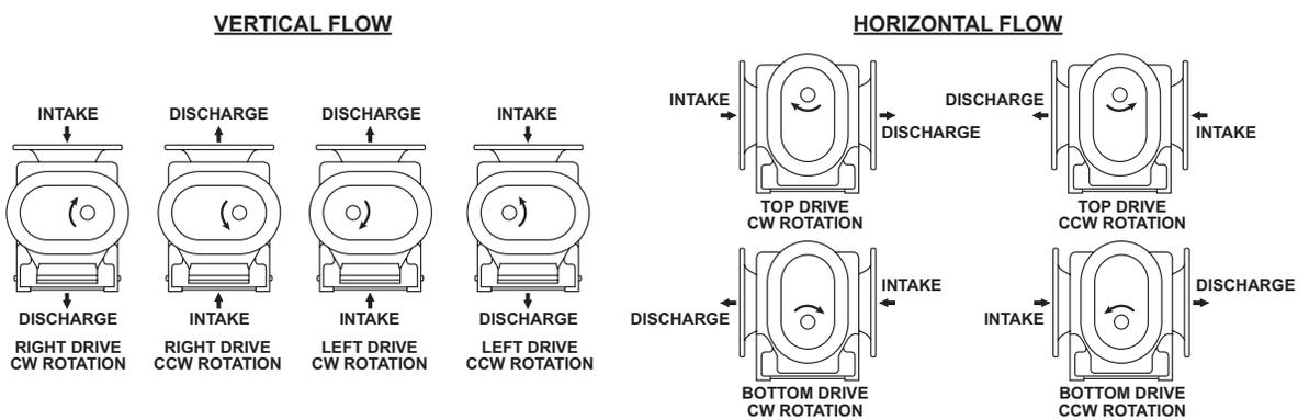
Figure 4-2 – Flow Direction by Rotation
