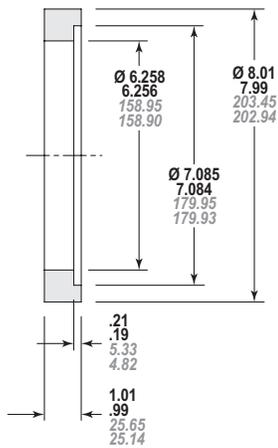
Figure 13-6 – Pilot Tool for Mechanical Seal
