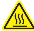
Do not touch hot surfaces. The upper limit of the blower operation is 400° F (205° C). Do not touch the blower while it is in operation and assure blower is cool when not in operation.
