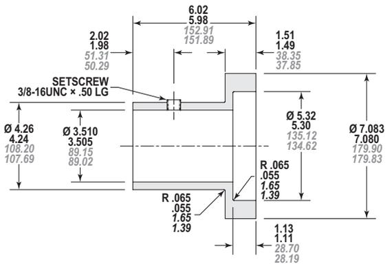
Figure 13-3 – Drive Shaft Bearing Alignment Tool
