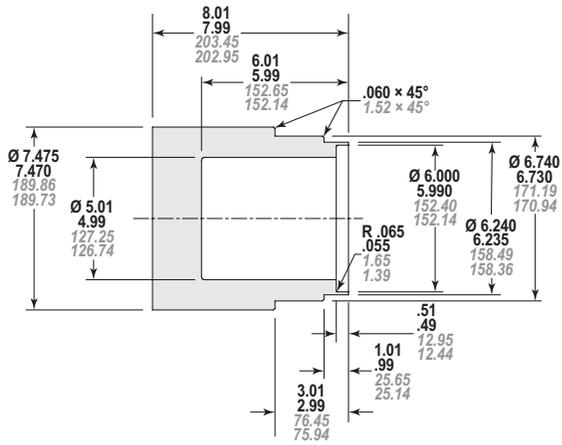
Figure 13-5 – Mechanical Seal Installation Tool
