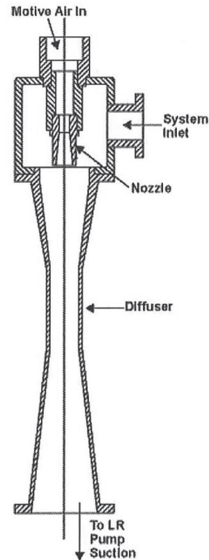
Figure 3-5 – Air Ejector
