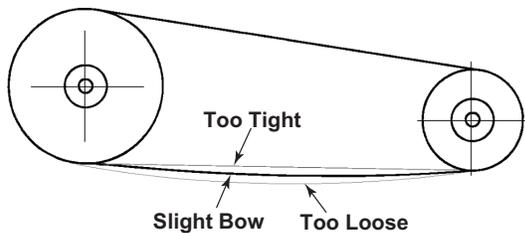
Figure 5-4 – General appearance of a V-belt drive
