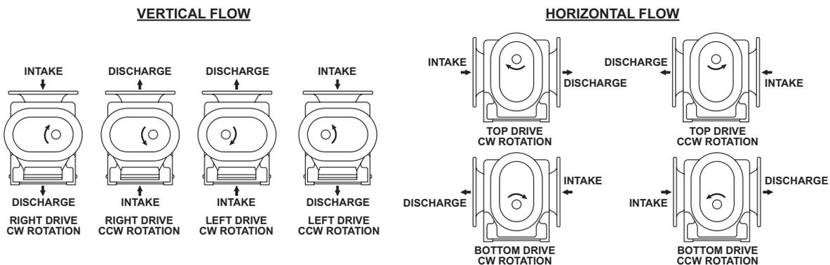
Figure 4-2 – Flow Direction by Rotation
