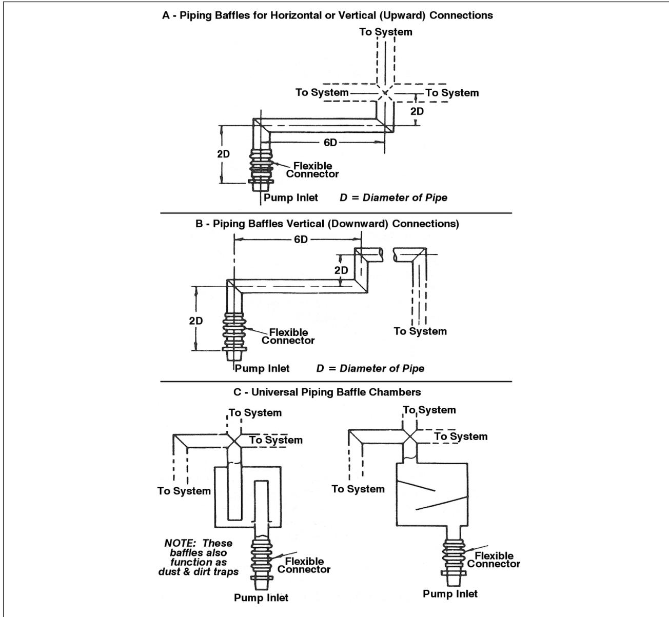
Figure 3-1 – Vacuum Manifolding with Integral Oil Baffles
