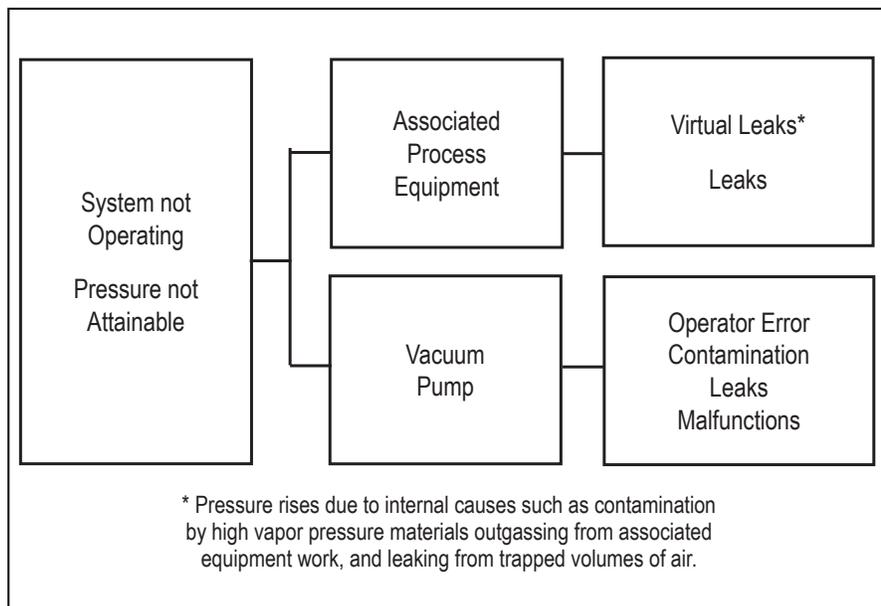
Figure 5-2 – Common Faults in Vacuum Systems
