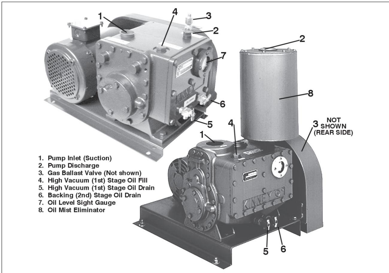
Figure 4-1 – Pump Components
