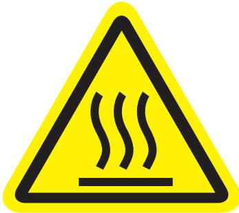
This label is placed at the process outlet. The outlet can approach temperatures as high as 400° F (204° C).
