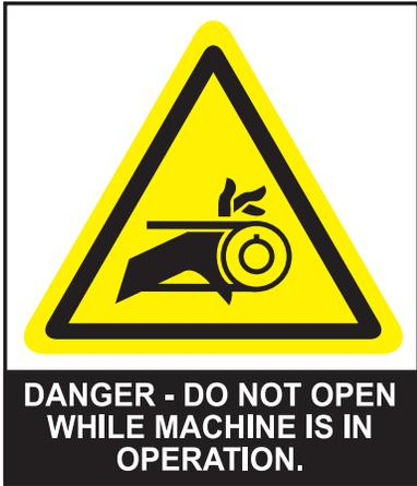
This label is placed on the front of the machine. The covers (doors) shall not be opened while the machine is in operation. Proper lock-out, tag-out procedures should be followed.
