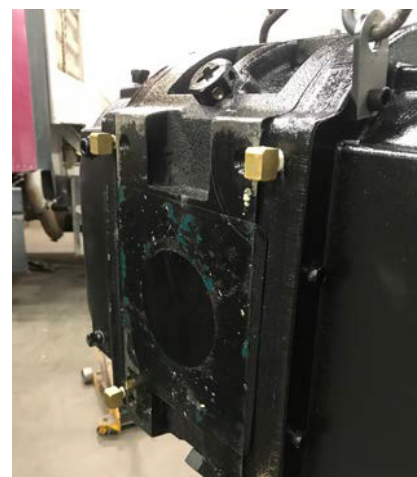
Figure 4-4 – Alternate plug configuration: Horizontal mount with street elbows
