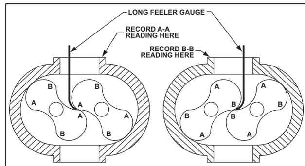
Figure 14 - Checking Rotor Interlobe Clearance
