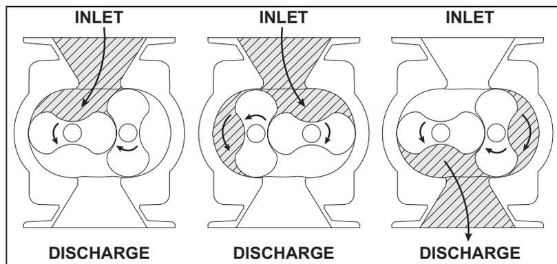
Figure 1 - Illustration of general operation principle
