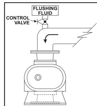
Figure 9 - Flushing Diagram
