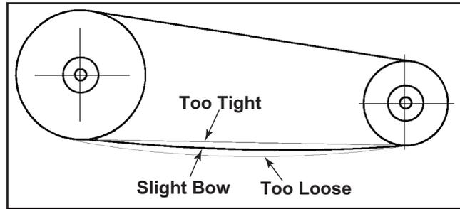
Figure 7 - General appearance of a V-Belt drive
