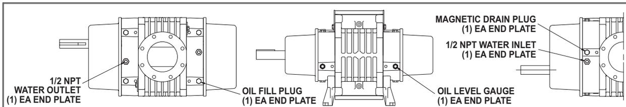
Figure 5 - Location of oil fill, drain, level gauges and cooling connections on boosters with water cooled endplates
