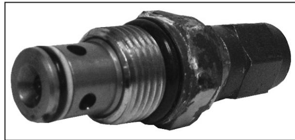
Figure 6 - Oil Pressure Adjustment Hex Cap
