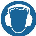
Noise emission. The highest noise pressure levels measured as per EN ISO 3744. When spending a long time in the vicinity of the running machine use ear protection to avoid permanent damage to your hearing.
