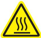
Hot surfaces. When the machine is at operating temperature the surface temperature on the components may go above 158°F (70°C). You must avoid touching the hot surfaces. These areas are marked with warning plates.
