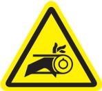
Internal and external rotating parts of the pump and driving equipment can produce serious physical injuries. The pump should never be run with the inlet or discharge piping removed. If it becomes necessary to inspect the rotating parts of the pump or to change the belt, be absolutely sure that all power to the motor controls has been shut off, the motor controls are locked out, and properly tagged before proceeding.
