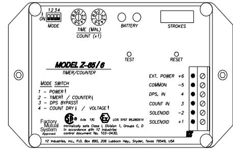
**1. Dry Contact Input:** mode switch 4 should be in the off position. Depress the test switch and hold. A red LED should illuminate. When the dry contact input is received at the counter input (ter. #3) the green LED will turn on and off and the red LED will illuminate again. This will normally occur very quickly and give the appearance that the green LED blinks on when the pulse input is received and removed.
