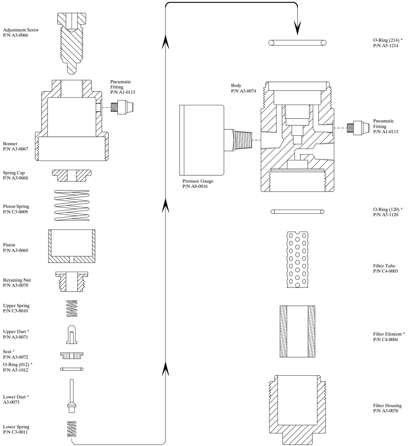
\* Filter/Regulator Repair Kit P/N D3-0003
