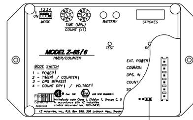
*Note: When the test is complete, move the jumper back to the factory position (far left position).*
