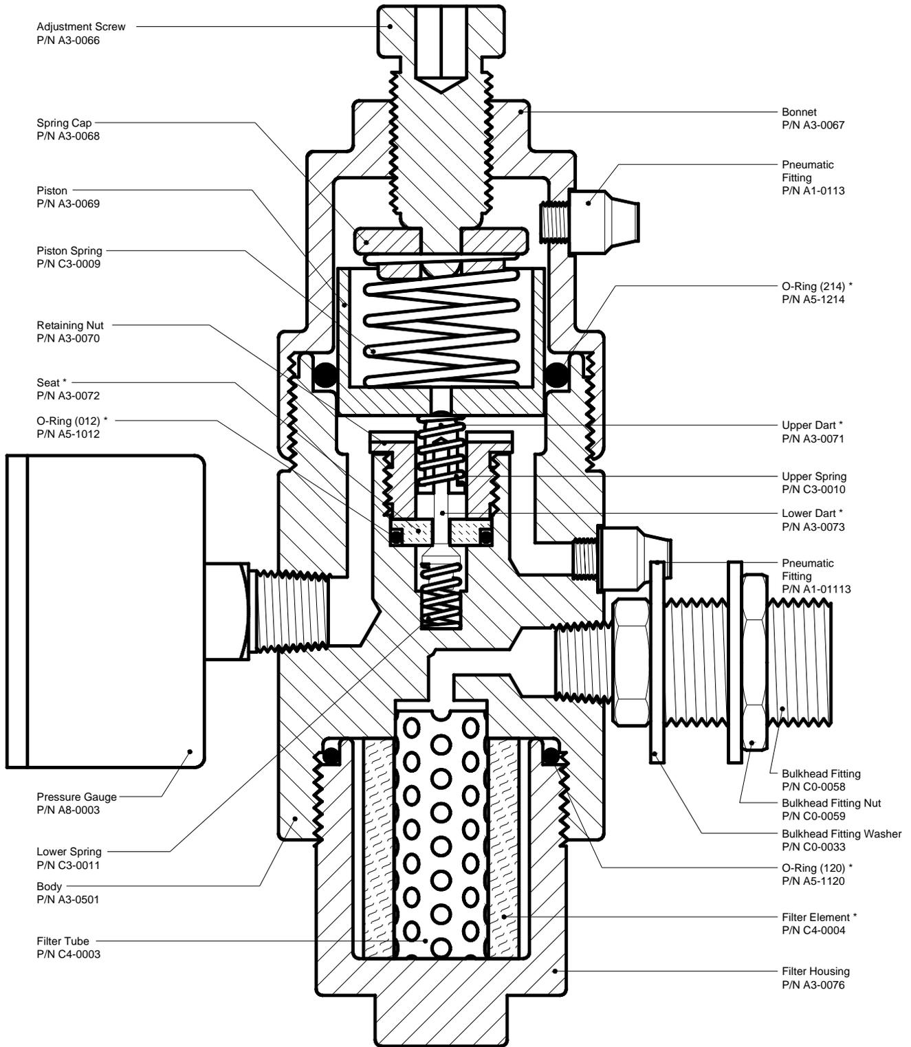
\* Filter/Regulator Repair Kit P/N D3-0116
