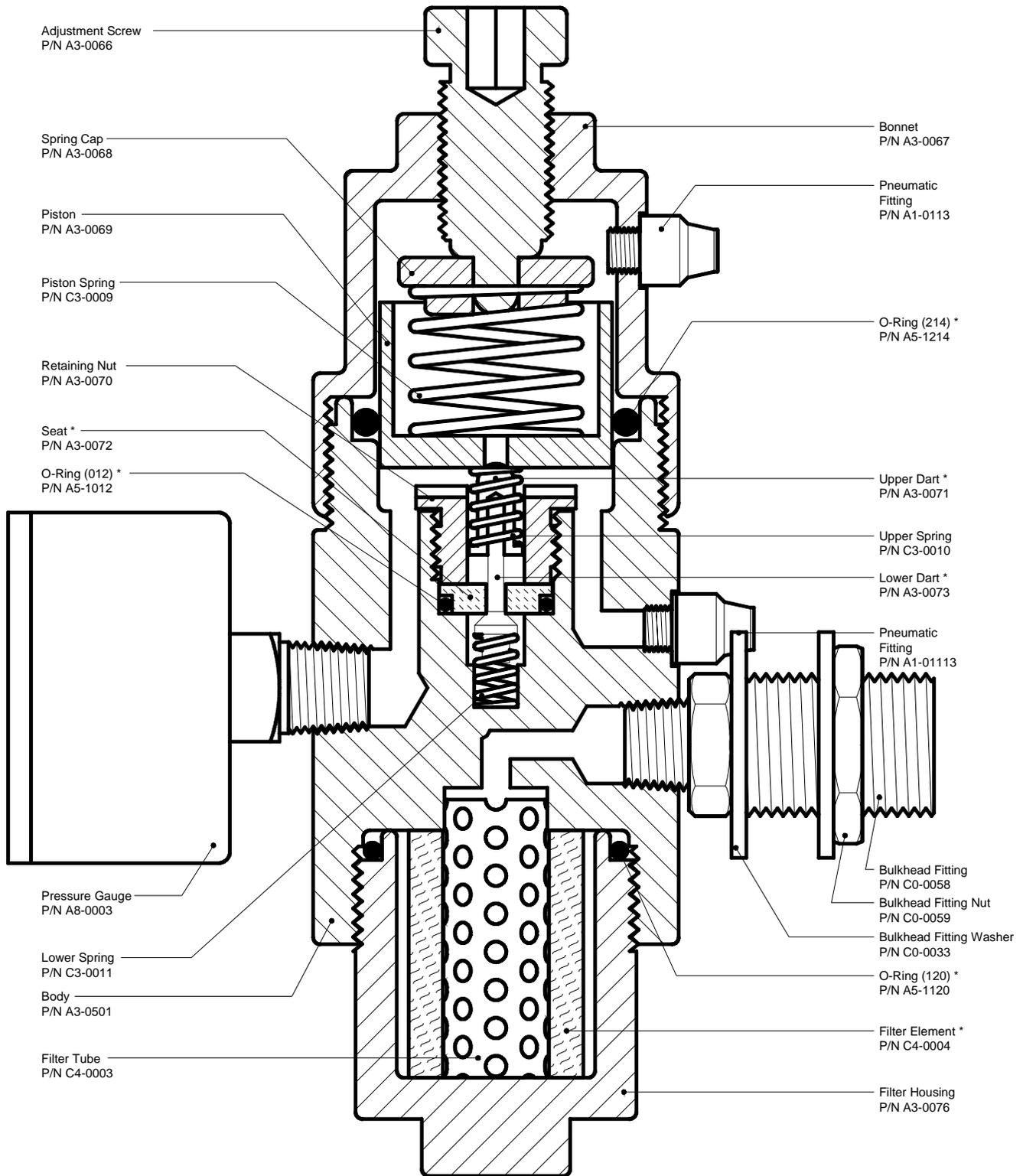
\* Filter/Regulator Repair Kit P/N D3-0116
