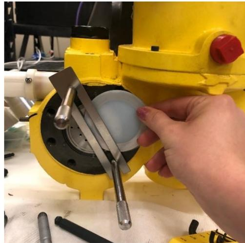
*Figure 62 Placing Diaphragms and Shims*
