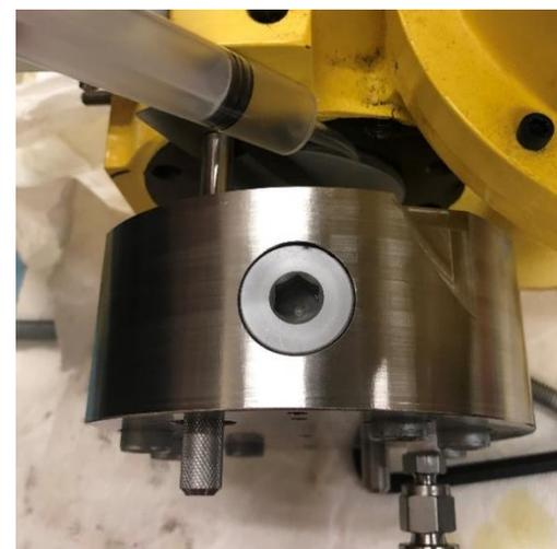
*Figure 66 Pump Head Prepared for Assembly while Injecting Mineral Oil*
