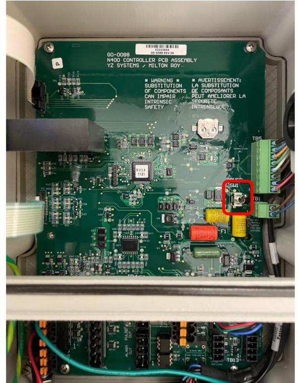
Figure 19 Controller board component layout with power switch location highlighted in a red rectangle.
