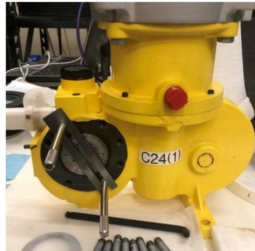
*Figure 63 Stud Tool with Diaphragm Retaining Tool Installed*
