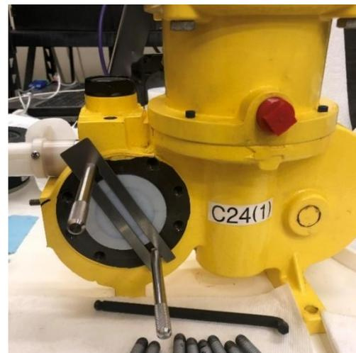
*Figure 64 Diaphragms and Shims Installed*
