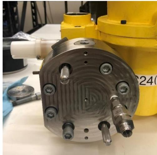
*Figure 65 Pump Head Prepared for Assembly with Diaphragm Retaining Tool Installed*
