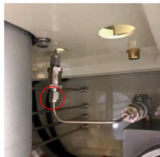
*Figure 67 Pressure Switch Line Fitting*
