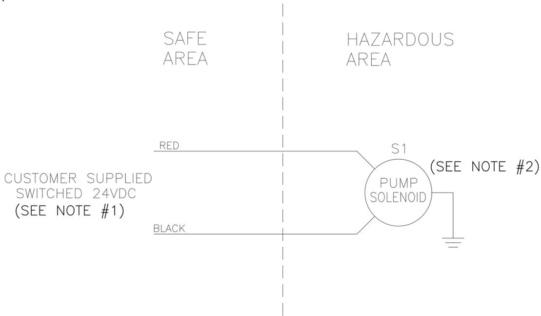
1. THE 24VDC SIGNAL MUST HAVE A MINIMUM DWELL OF 3 SECONDS.
