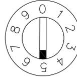
B. Set the data switches to 00.0 to enter the diagnostic mode of operation.
