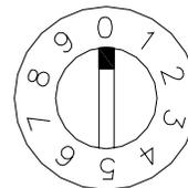
**NOTE:** Time (20.0 minutes) above corresponds to dial setting shown for the Z-200.1 model. (For the Z-200.10, the time would be 2.00 minutes - the decimal moves one place to the left).
