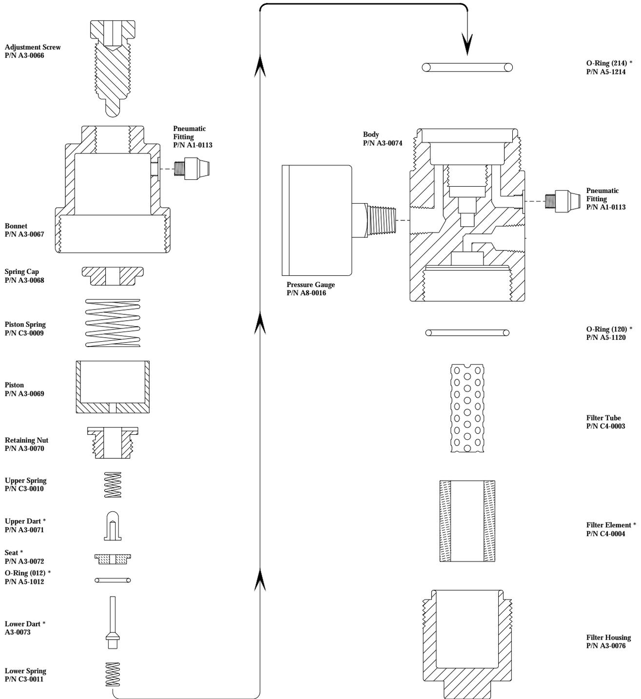
\* Filter/Regulator Repair Kit P/N D3-0003
