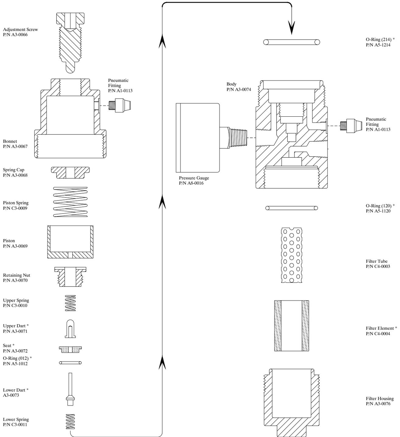
\* Filter/Regulator Repair Kit P/N D3-0003
