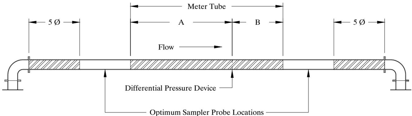
A = The number of unobstructed, straight pipe diameters upstream (see AGA - 3 manual).
