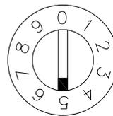
9.2 Adjust the pump volume adjustment knob to the value used in the calculations in step 9.1.
