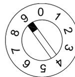
7.10 Return the mode switch to position 9 (off position).
