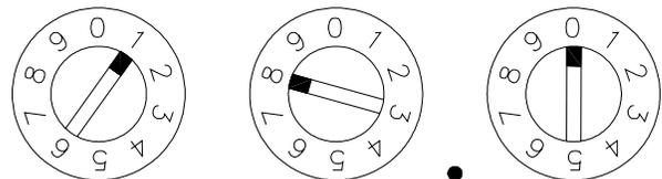
*NOTE: Time (18.0 minutes) above corresponds to dial setting shown for the Z-200.1 model. (For the Z-200.10, the time would be 1.80 minutes - the decimal moves one place to the left).*
