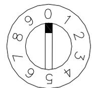
**NOTE:** Time (20.0 minutes) above corresponds to dial setting shown for the Z-200.1 model. (For the Z-200.10, the time would be 2.00 minutes - the decimal moves one place to the left).
