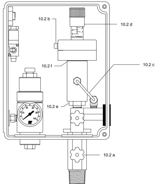
*NOTE: normal service generally requires only the replacement of the o-rings and seal. A seal repair kit (part number D3-0002) is available from YZ.*
