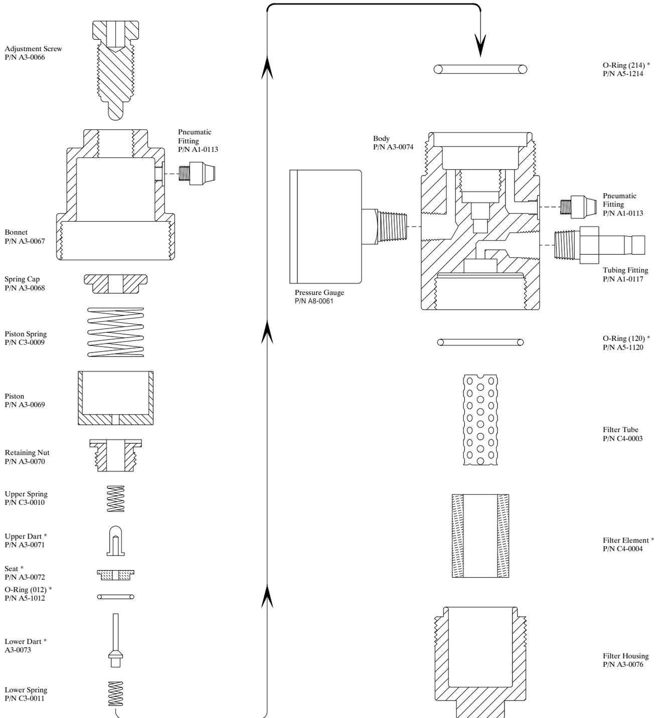
\* Filter/Regulator Repair Kit P/N D3-0003
