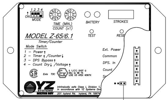
**NOTE:** When the test is complete, move the jumper back to the factory position (far left position).
