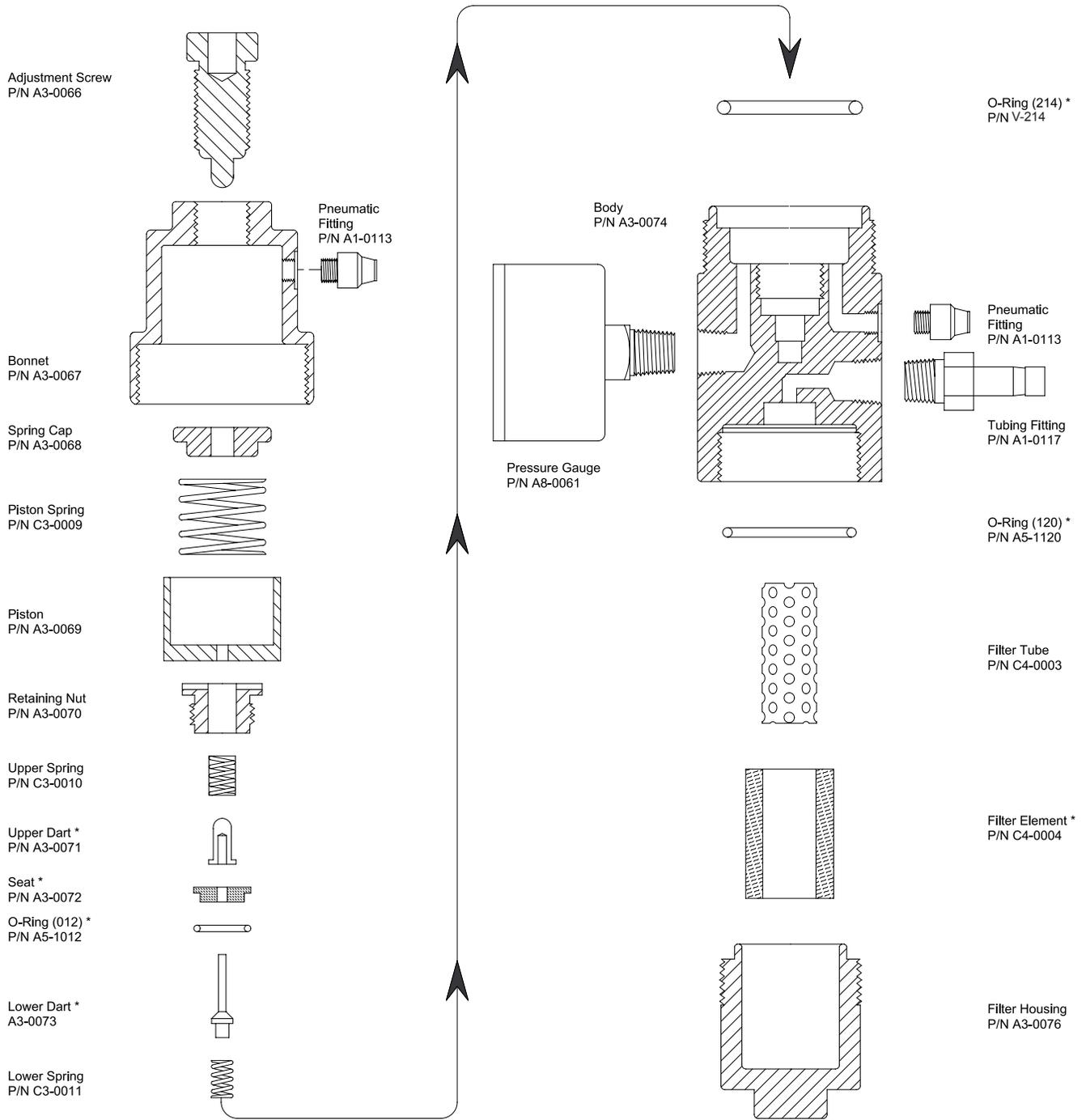
\* Filter / Regulator Repair Kit P/N D3-0003
