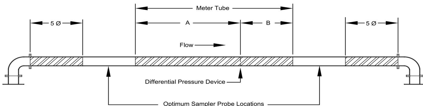
A= The number of unobstructed, straight pipe diameters upstream (see AGA – 3 manual).
