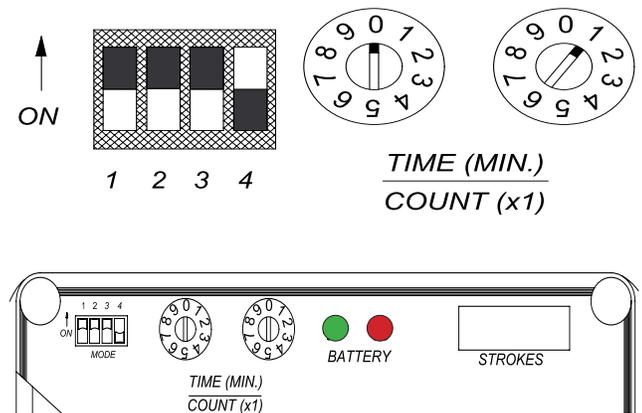
**NOTE:** Time switches must not be in 00 position to test the battery.
