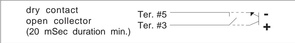
**2. Voltage Pulse Input:** move mode switch 4 to the on position. Depress the test switch and hold. A green LED should illuminate. When the voltage pulse input is received at the count input (ter. #3) the red LED will turn on and off and the green LED will illuminate again. This will normally occur very quickly and give the appearance that the red LED blinks on when the pulse input is received and removed.
