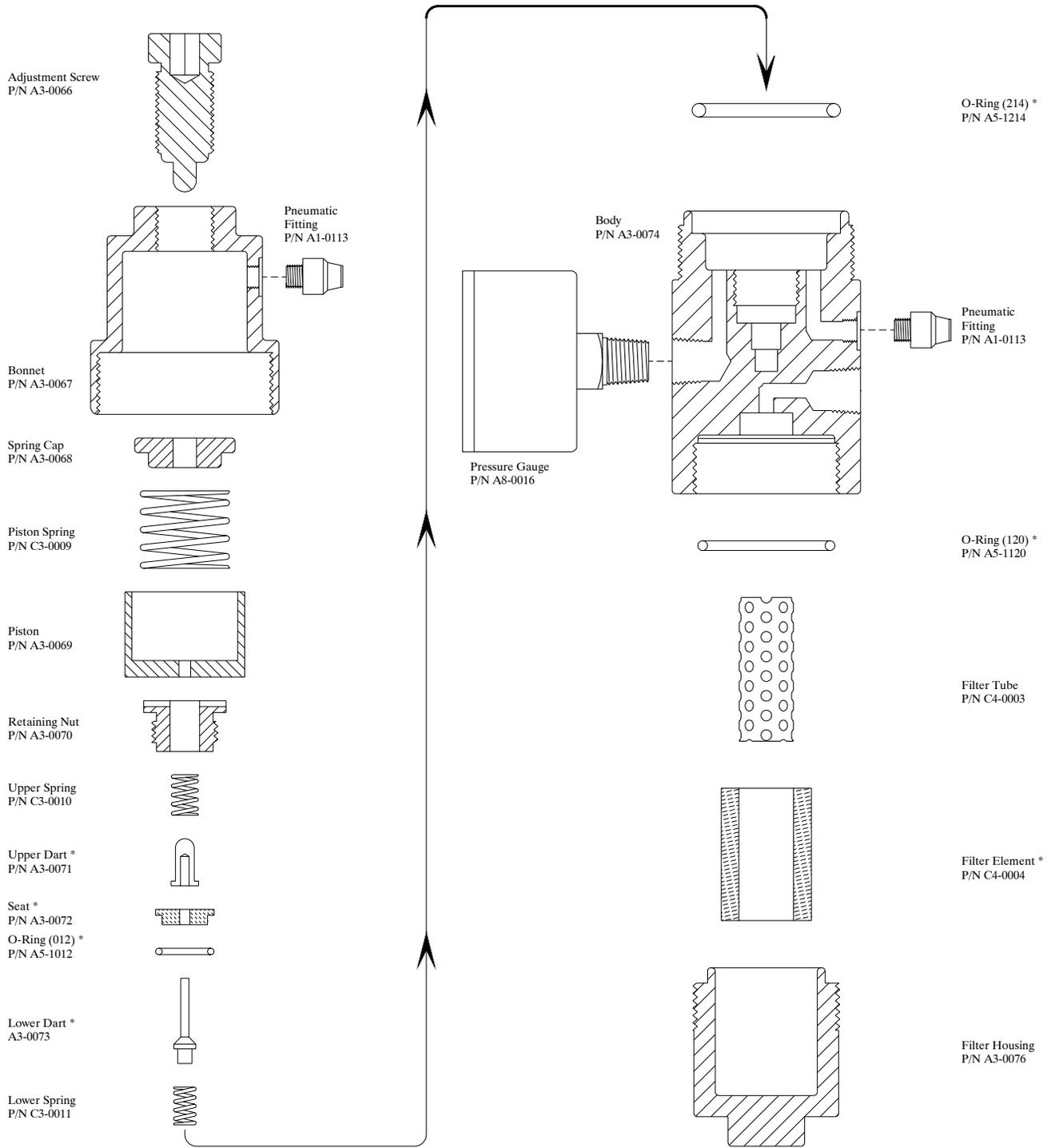
\* Filter/Regulator Repair Kit P/N D3-0003
