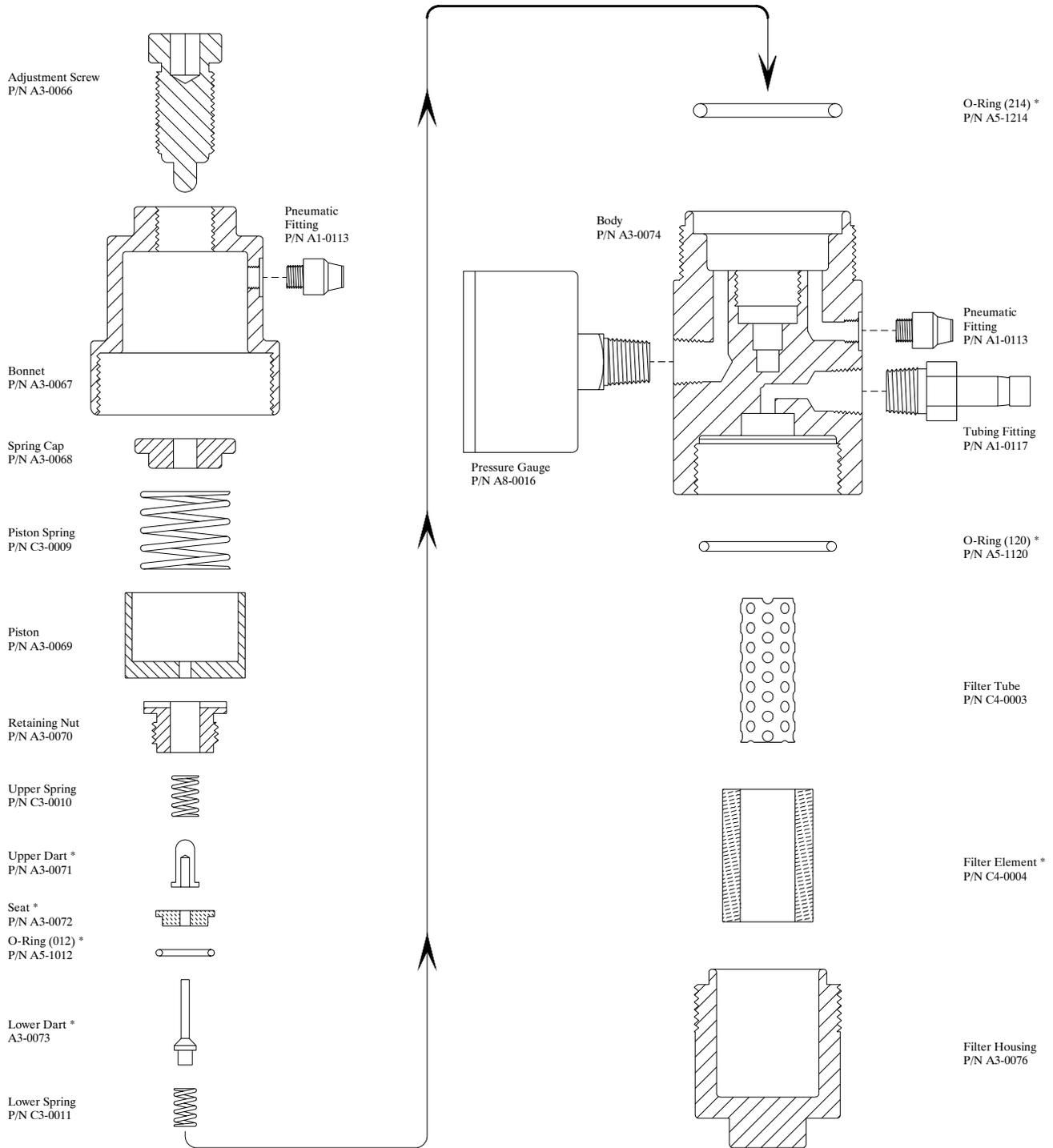
\* Filter/Regulator Repair Kit P/N D3-0003
