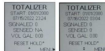
**PUMP ALARM SCREEN (610F only):** If your system has a flow switch from the home screen, the pump alarm screen can be accessed by pressing the navigation switch twice in the down direction. The pump alarm screen shows the number of strokes signaled (sent to the pump) and how many strokes were sensed (counted by the flow switch).
