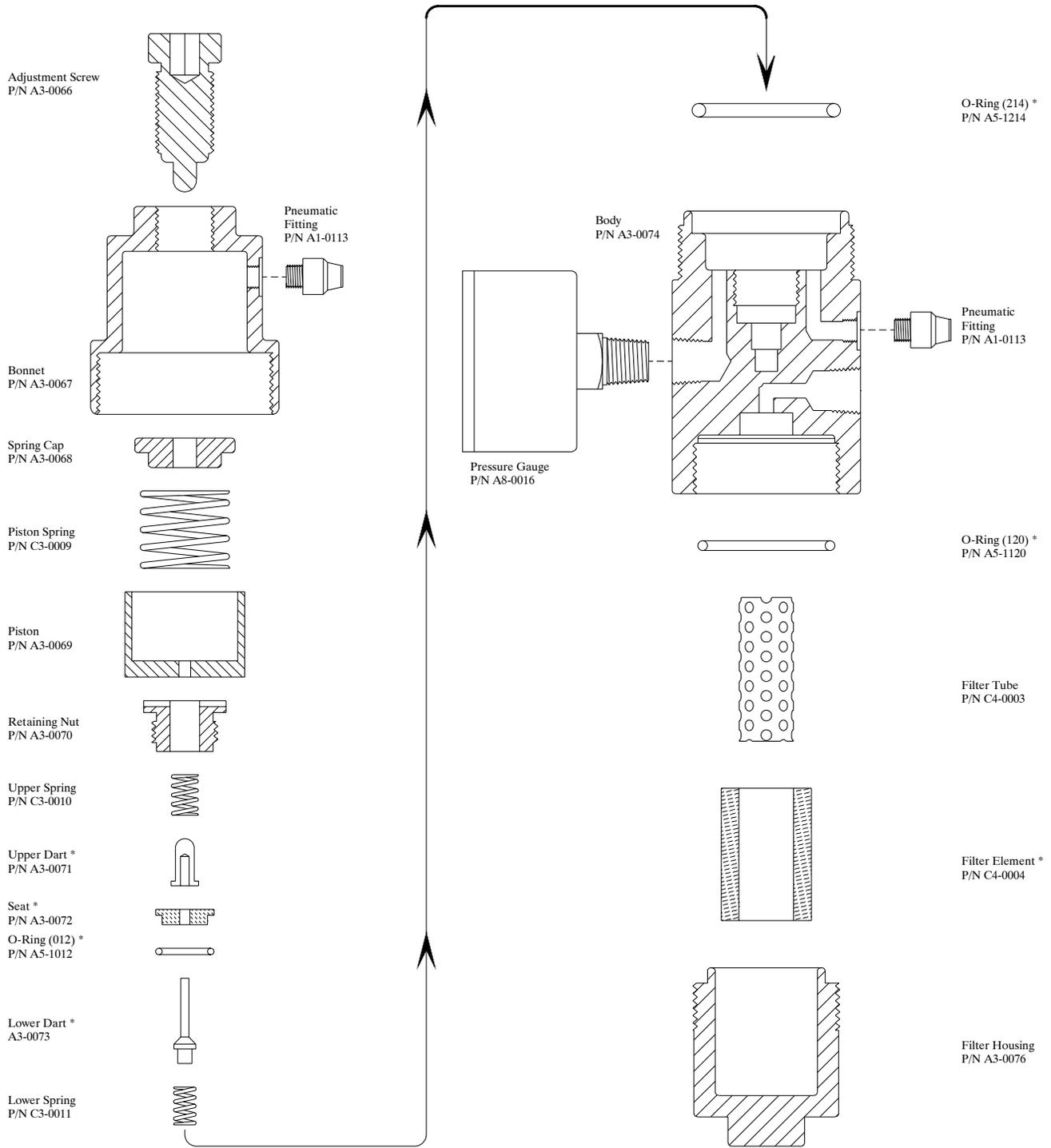
\* Filter/Regulator Repair Kit P/N D3-0003
