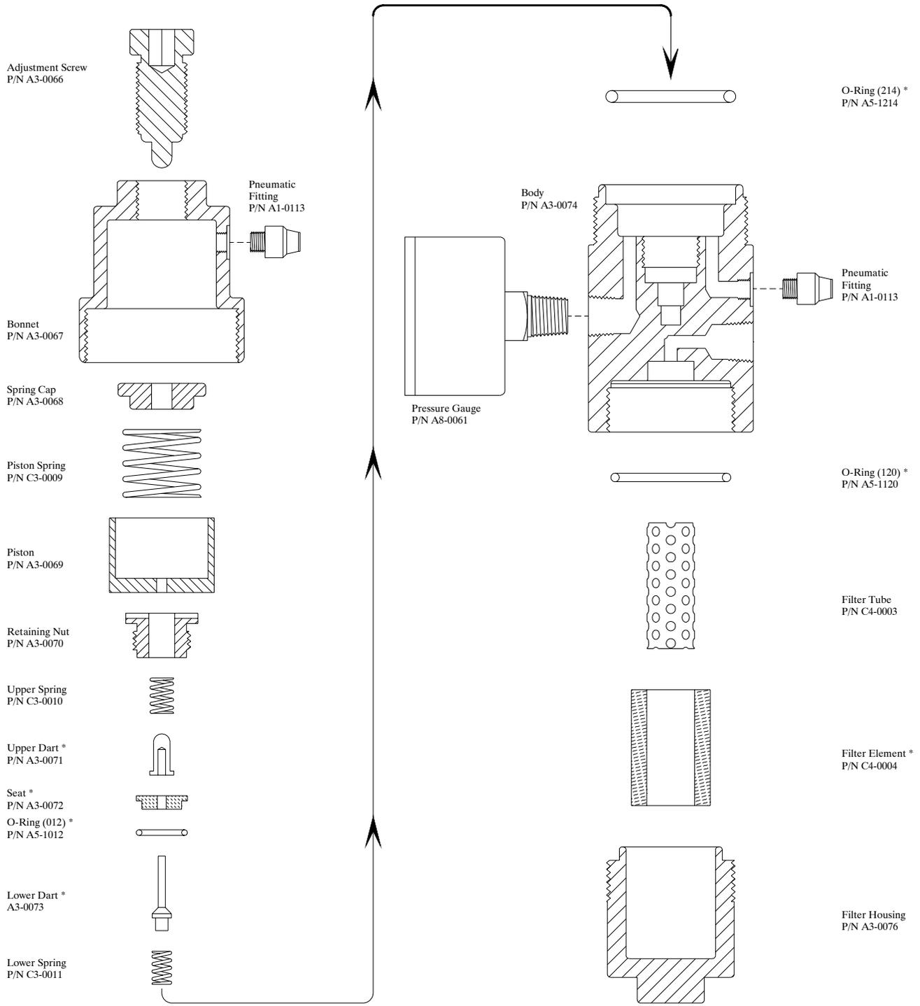
\* Filter/Regulator Repair Kit P/N D3-0003
