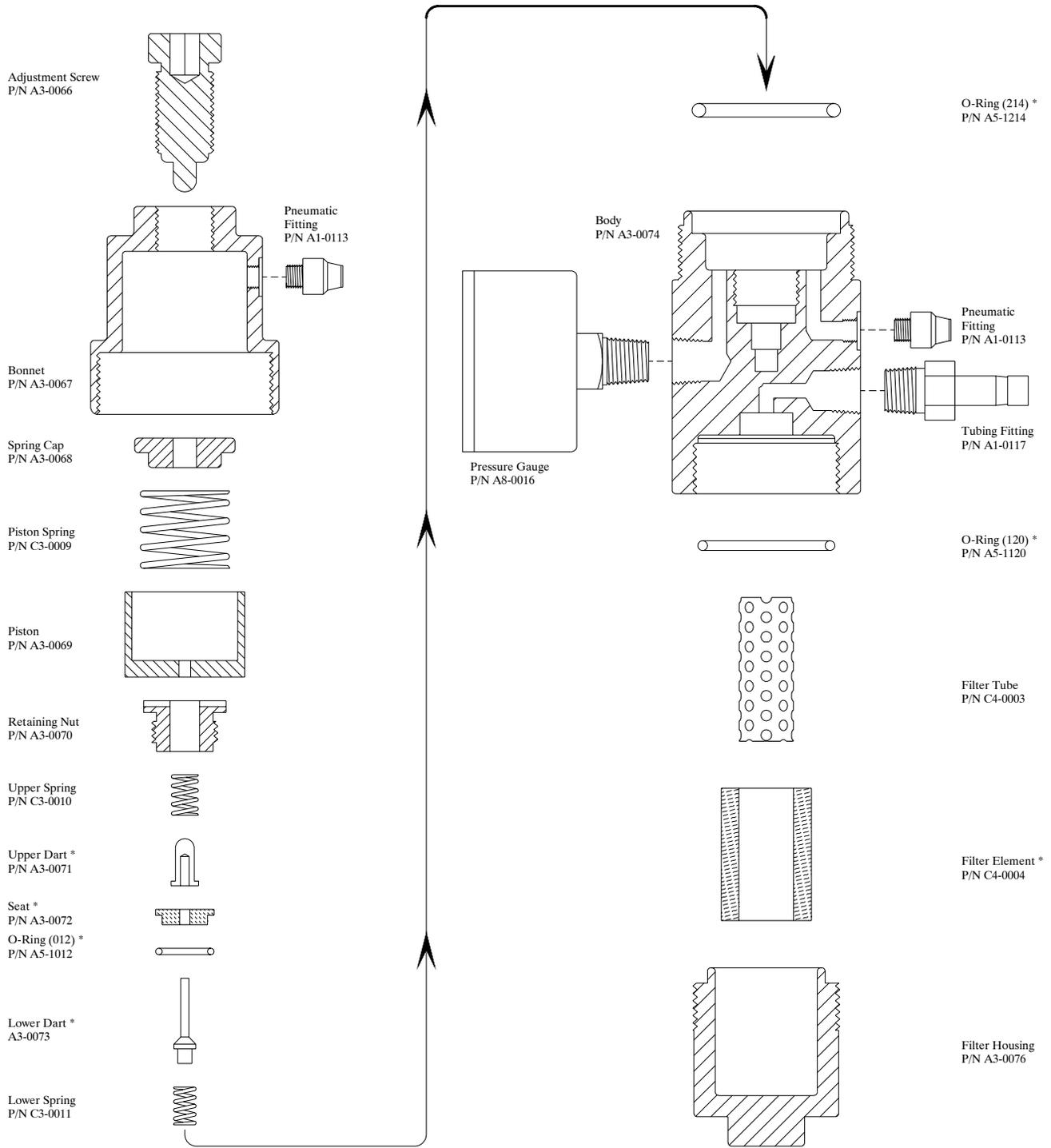
\* Filter/Regulator Repair Kit P/N D3-0003
