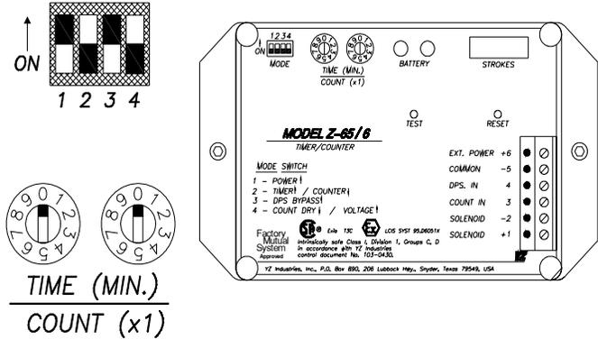
**1. Dry Contact Input:** mode switch 4 should be in the off position. Depress the test switch and hold. A red LED should illuminate. When the dry contact input is received at the counter input (ter. #3) the green LED will turn on and off and the red LED will illuminate again. This will normally occur very quickly and give the appearance that the green LED blinks on when the pulse input is received and removed.
