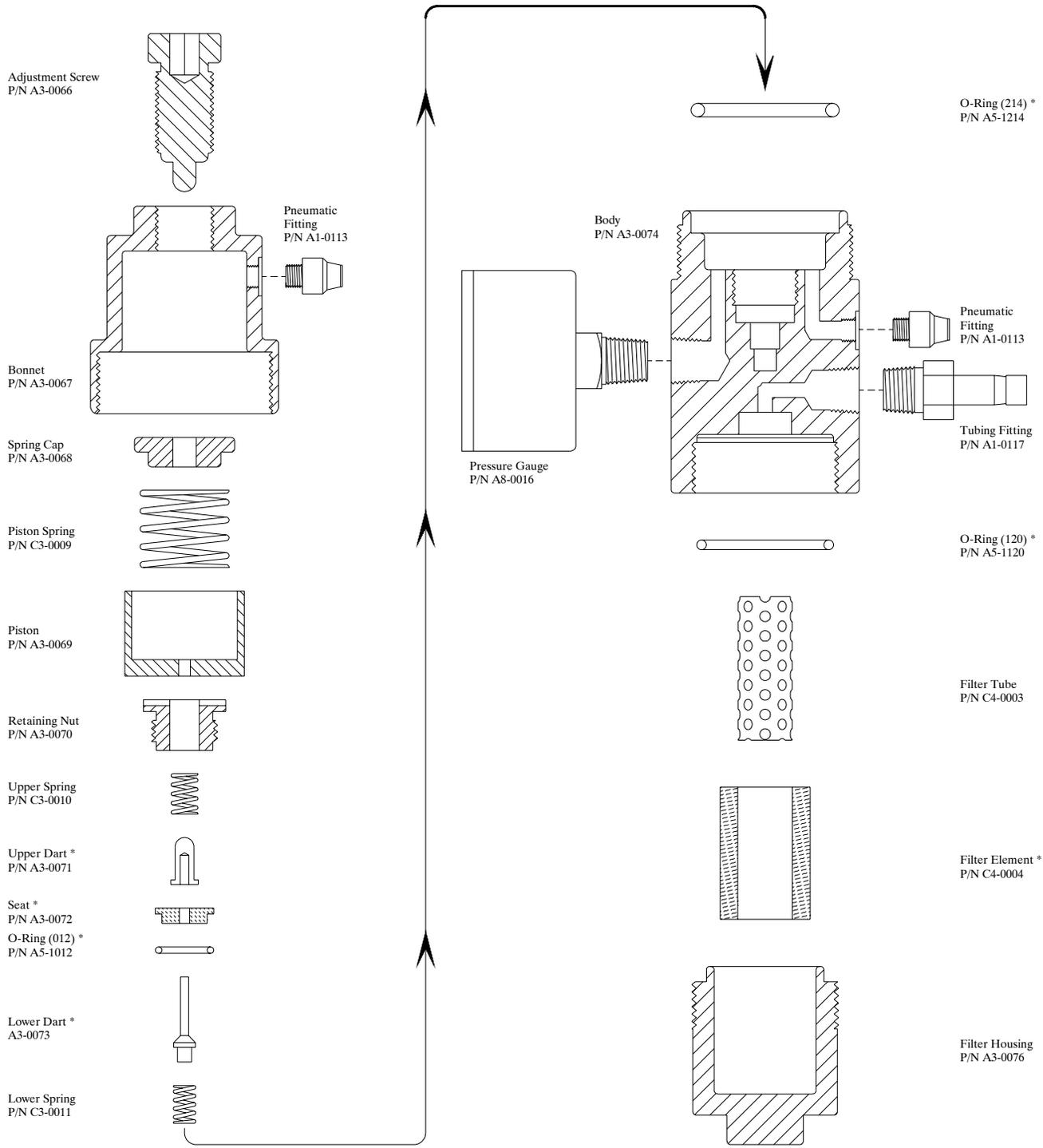
\* Filter/Regulator Repair Kit P/N D3-0003
