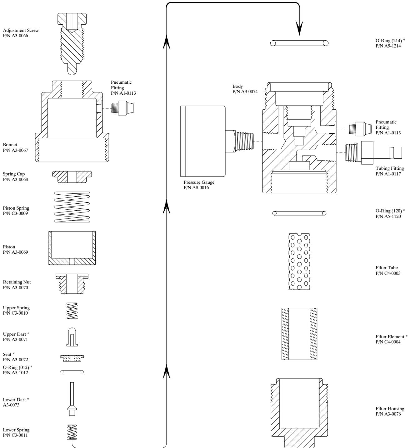
\* Filter/Regulator Repair Kit P/N D3-0003
