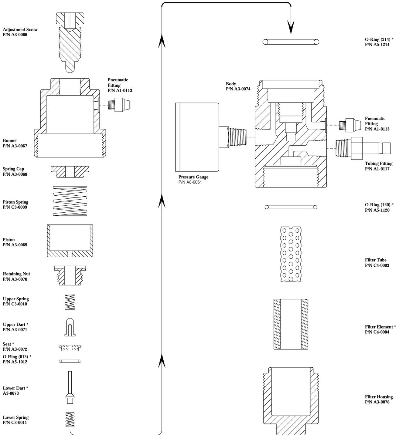
\* Filter/Regulator Repair Kit P/N D3-0003
