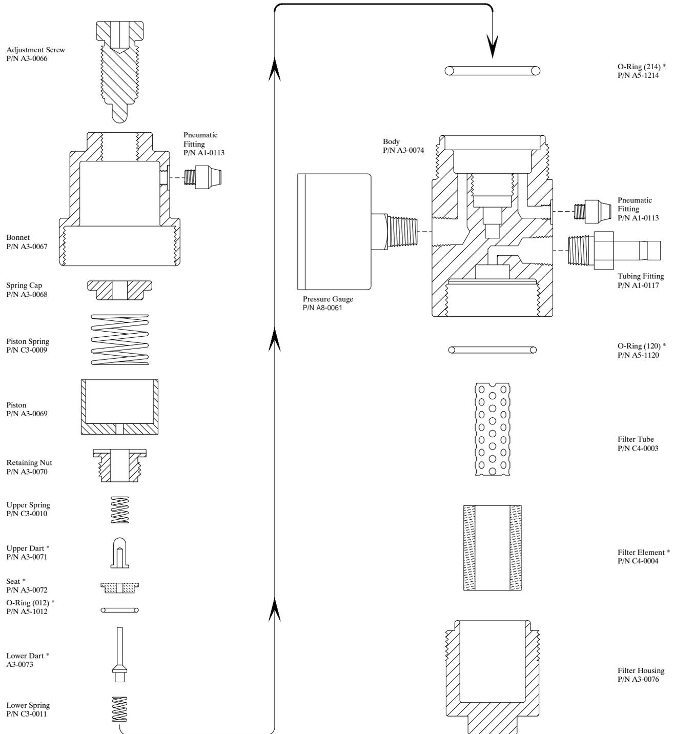
\* Filter/Regulator Repair Kit P/N D3-0003
