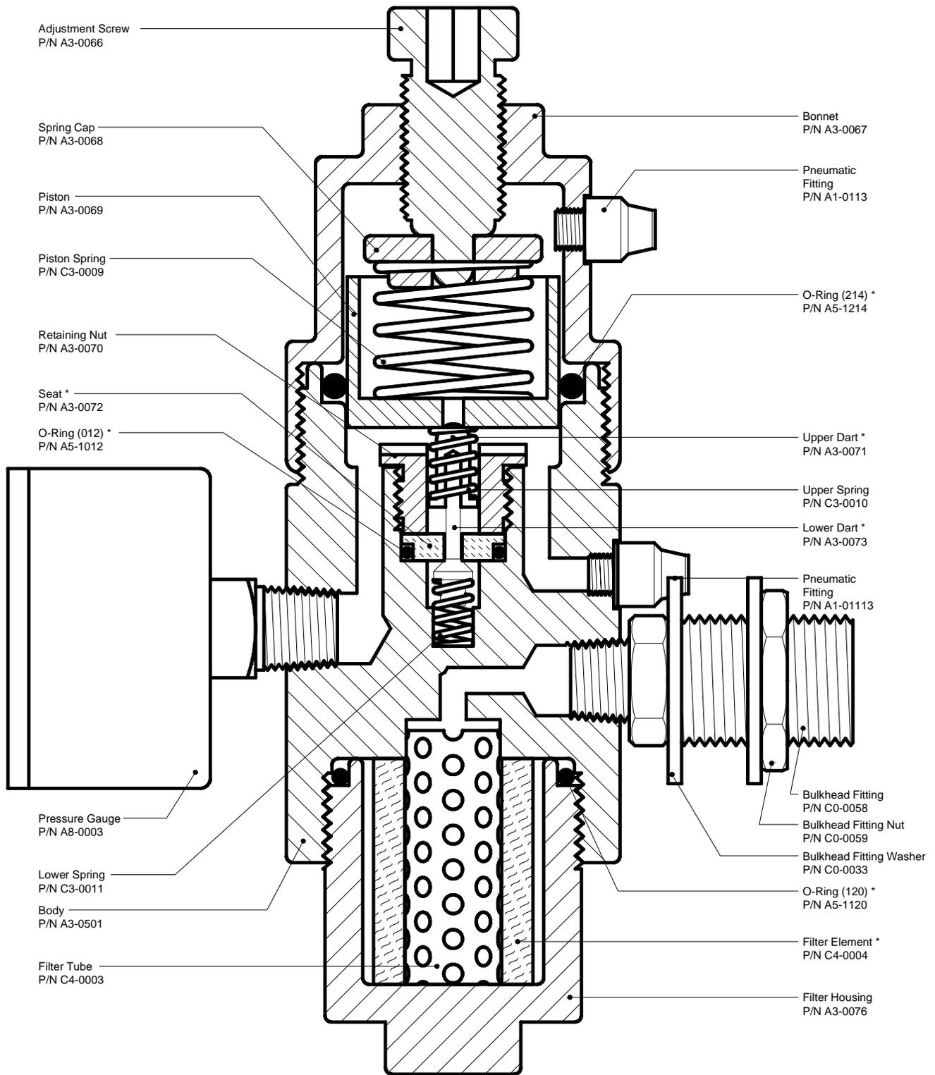
\* Filter/Regulator Repair Kit P/N D3-0116
