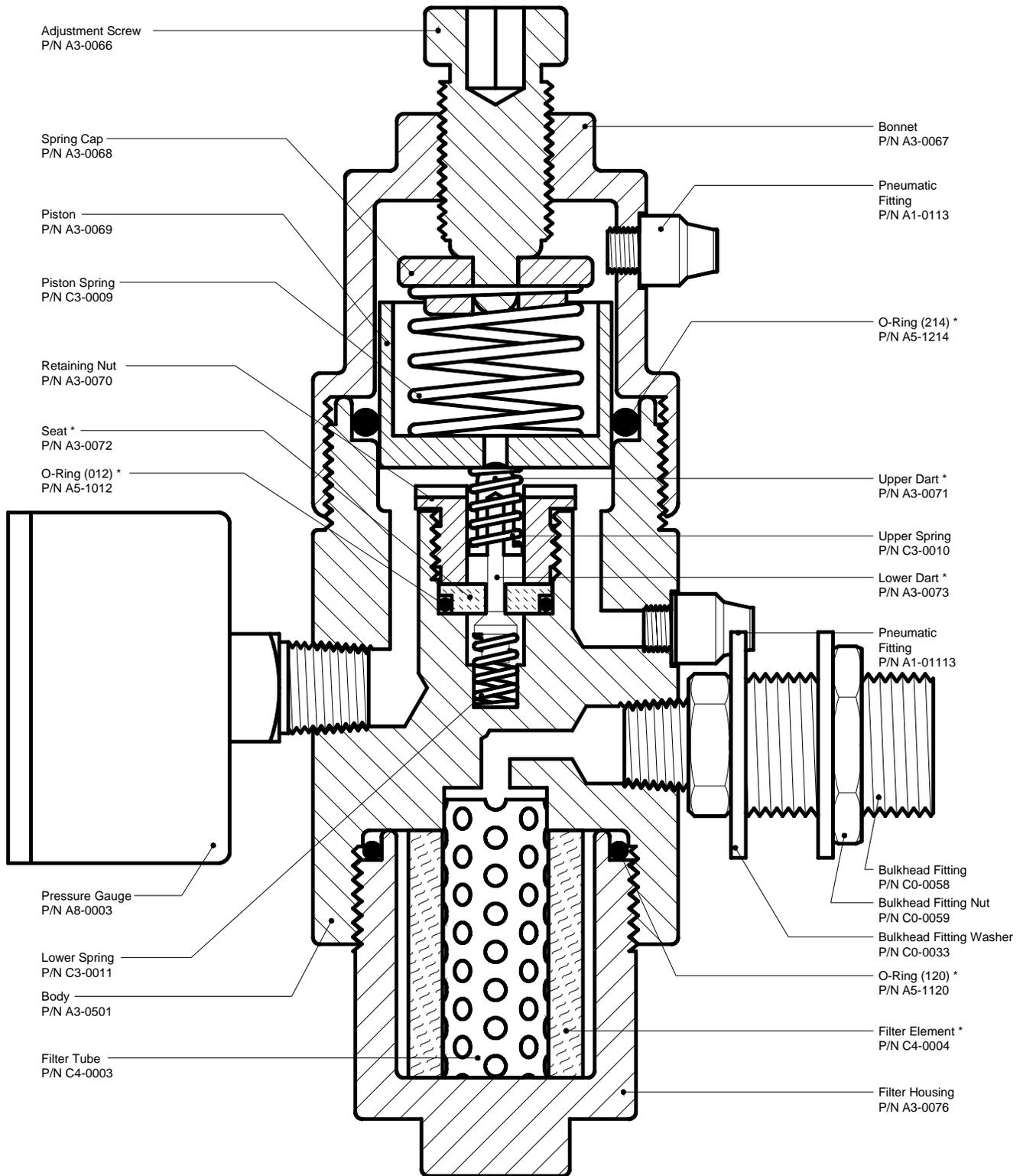
\* Filter/Regulator Repair Kit P/N D3-0116
