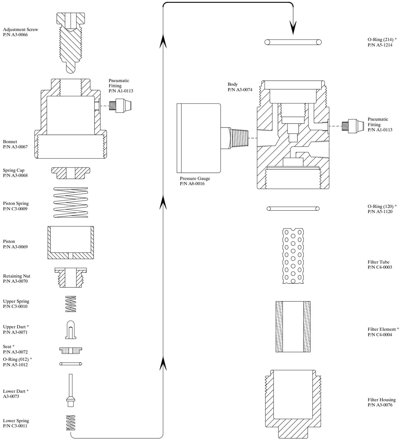
\* Filter/Regulator Repair Kit P/N D3-0003
