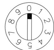
**NOTE:** Time (18.0 minutes) above corresponds to dial setting shown for the Z-200.1 model. (For the Z-200.10, the time would be 1.80 minutes - the decimal moves one place to the left).
