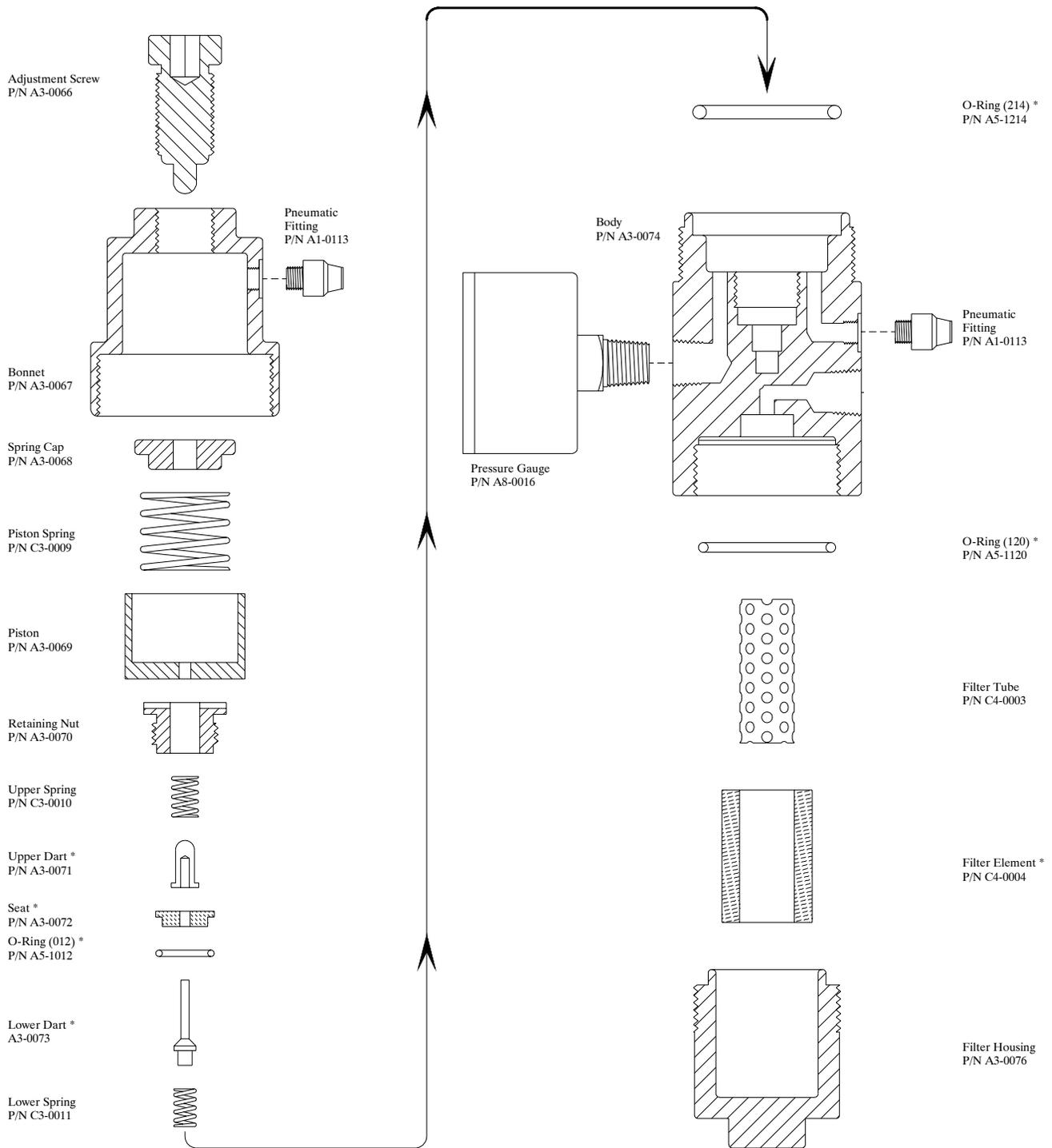
\* Filter/Regulator Repair Kit P/N D3-0003
