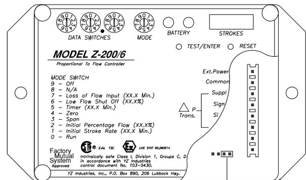
Setting for stroke indicator test configuration jumper
