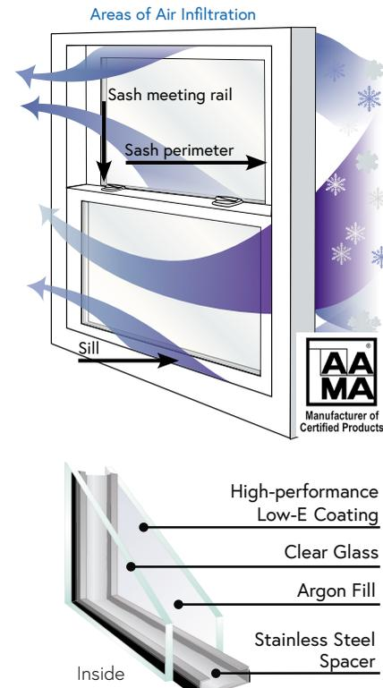
The Barrington window comes standard with one of our double-pane, high-performance Low-E glass systems with a stainless steel spacer, which will help to dramatically improve the efficiency of your new windows.
