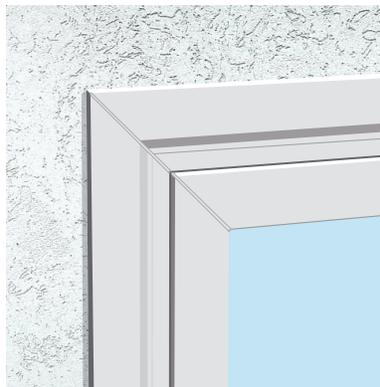
This replacement window configuration comes with a flange on the exterior of the window to cover and seal the frame on home with stucco.
