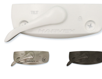
Dual-action locks allow you to lock or tilt open the window with a flip of the thumb. Double low-profile sash locks come in three different finishes - white, oil-rubbed bronze, and brushed nickel
