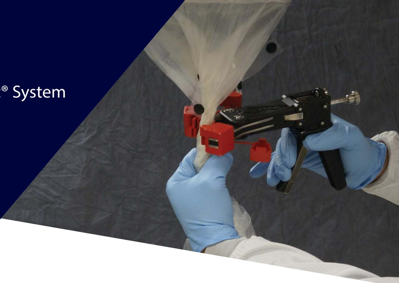
ILC Dover pioneered flexible containment for the pharmaceutical industry and continues to innovate processes for better performance. We invented the original CrimpLoc™ System to provide high containment and a secure closure when using the ILC Dover Continuous Liner, and other ArmorFlex® film solutions.
