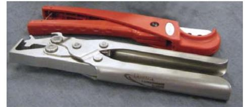
Crimp Removal Tool - The latest innovation for safe removal of the crimp. The crimp remains in one piece so no risk of contamination upon opening.
