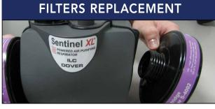
1. After Decon, turn filters counterclockwise. Unscrew filters and discard. Before installing new filter check gasket for any damage.
