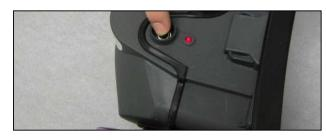
5. Depress switch on top of blower. A short beep should sound and light the red LED continuously. Audible beeping and blinking red LED light indicates low battery. Leave contaminated area and recharge.
