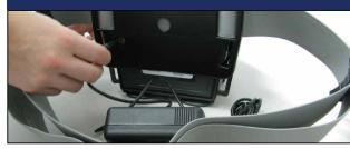
1. Plug battery charger into socket at back of the battery pack and connect to an electrical outlet. Charge battery pack for approximately five hours before use. The battery charger LED will flash green when charging is complete.
