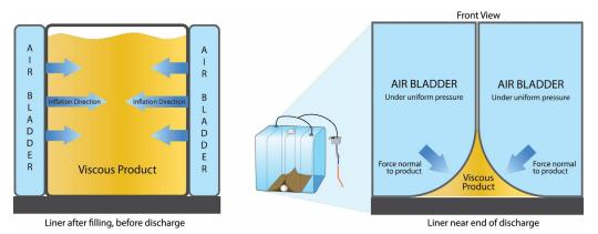
As the product is pumped from the IBC, an air bladder on each side of the liner inflates to fill the corners of the IBC and push the product towards the discharge port. This reduces the cavitation near the discharge port that occurs with viscous liquids and standard form-fit or pillow liners. Liquid is continuously presented to the discharge port without continuous manual manipulation.
